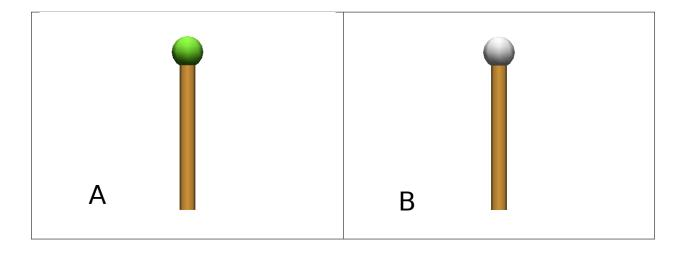
The **SetColor** primitive allow you to specify the appearance of the next primitive drawn by the turtle using either an index in the **Color Map** or directly using **red**, **green**, **blue** (or rgba) values as arguments (Fig. B). It is also possible to pass directly a plantgl **Material** object to specify a more complex appearance.
